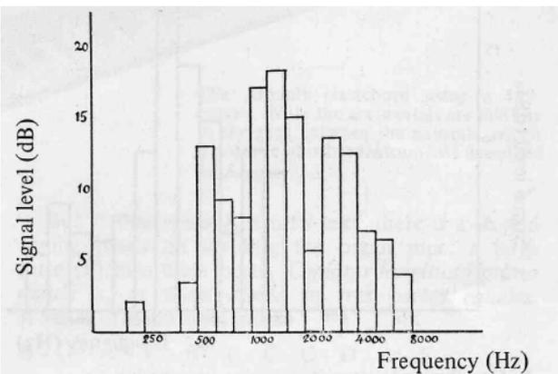
3. Third-octave bandwidth frequency analysis of the starting transient of a note produced with a leather plectrum (a) before wear and (b) after 1½ hours wear.
